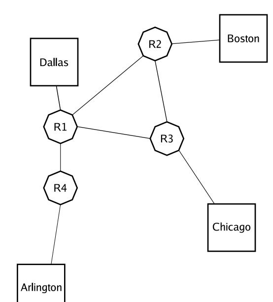
The Internet does not require each host to know how to reach another host, only the address of the host to reach. The network routers find a path by which to deliver each packet.
